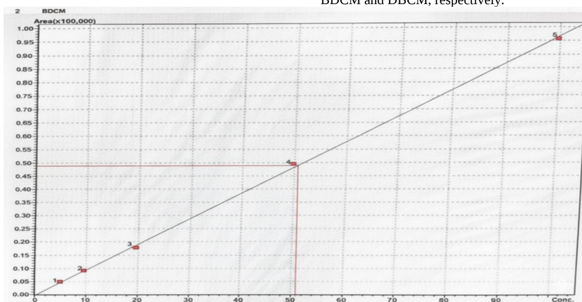
Fig. 5. Calibration curve of BDCM by new preconcentration method based on Headspace-GC-FID.
