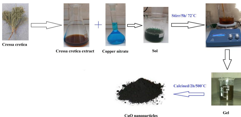
Fig. 1. Schematic of the synthesis of CuO nanoparticles
