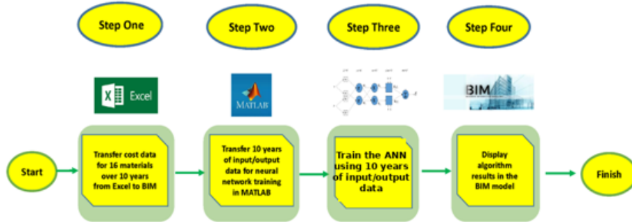
Figure 7: Workflow of ANN implementation in the BIM model
