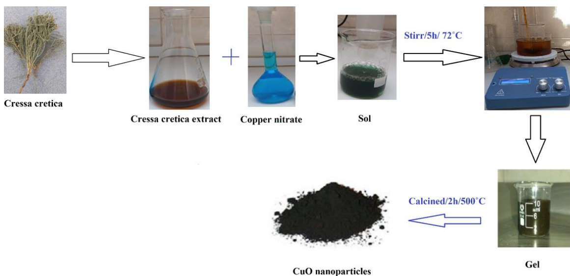
Fig. 1. Schematic of the synthesis of CuO nanoparticles
